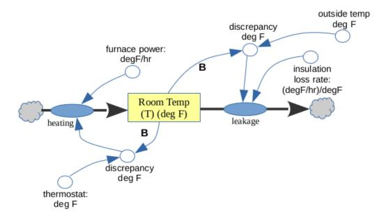
There are two balancing loops, one of which is "trying" to get the T stock to be equal to the thermostat setting, and the other of which is "trying" to get it to be the outside temperature.
